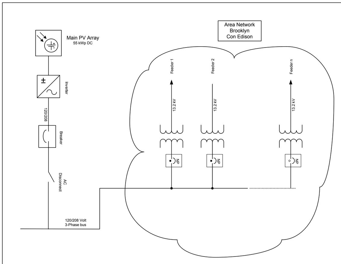
**Figure 14. Simplified Electrical One-Line Diagram for GMDC**
