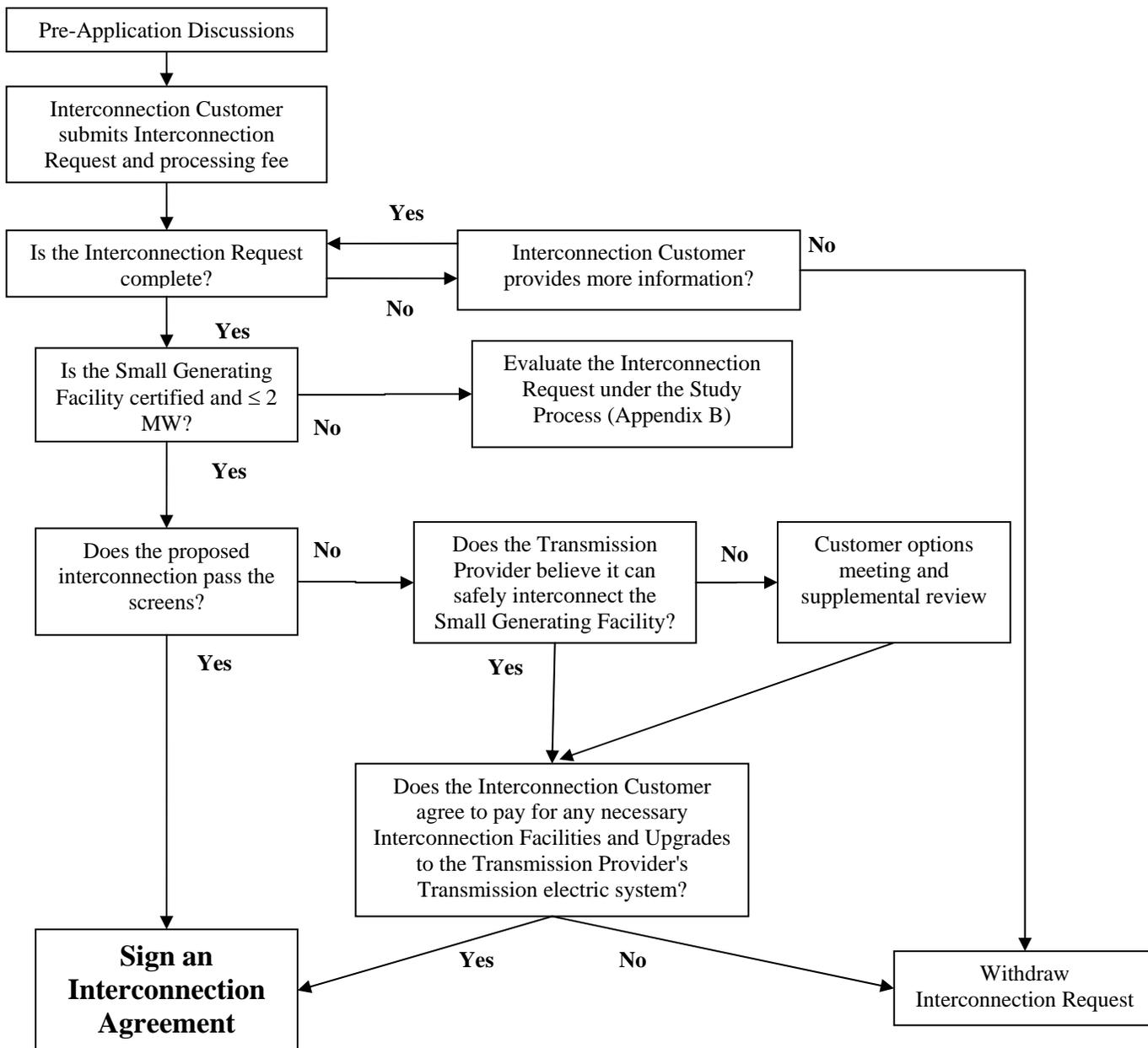
**Flow Chart for Interconnecting a Certified Inverter-Based
